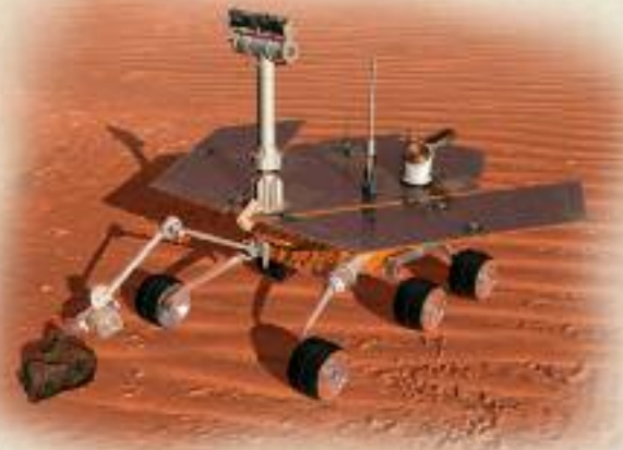
The twin rovers, Spirit and Opportunity, landed on Mars in 2004, and were still operating in 2011. Powered by solar panels, each rover was equipped with cameras and a robotic arm.
